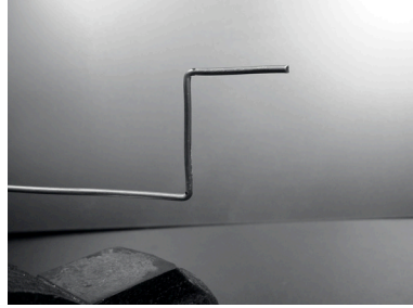
Figure 4.17: Bend the wire into a "Z" shape.
