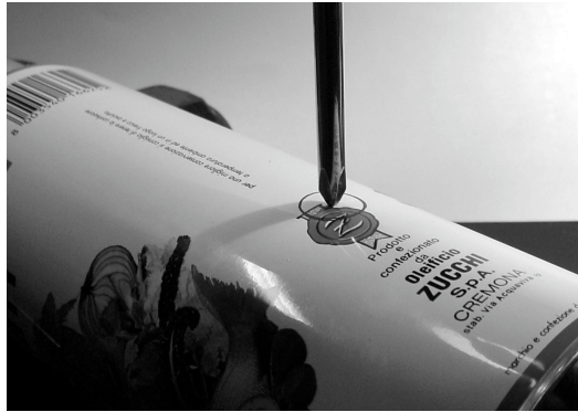
Figure 4.36: Mark the hole before drilling.
