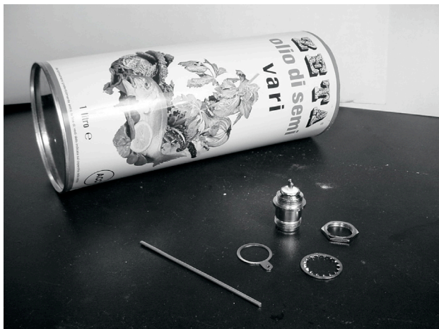
Figure 4.34: Parts needed for the can antenna.
