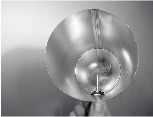
Figure 4.42: Your finished cantenna.
