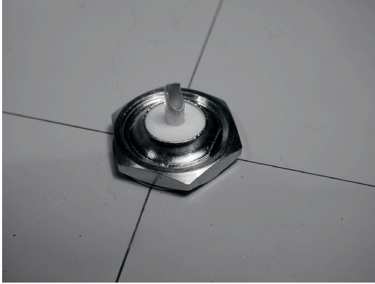
Figure 4.25: Secure the N connector tightly to the plate.
