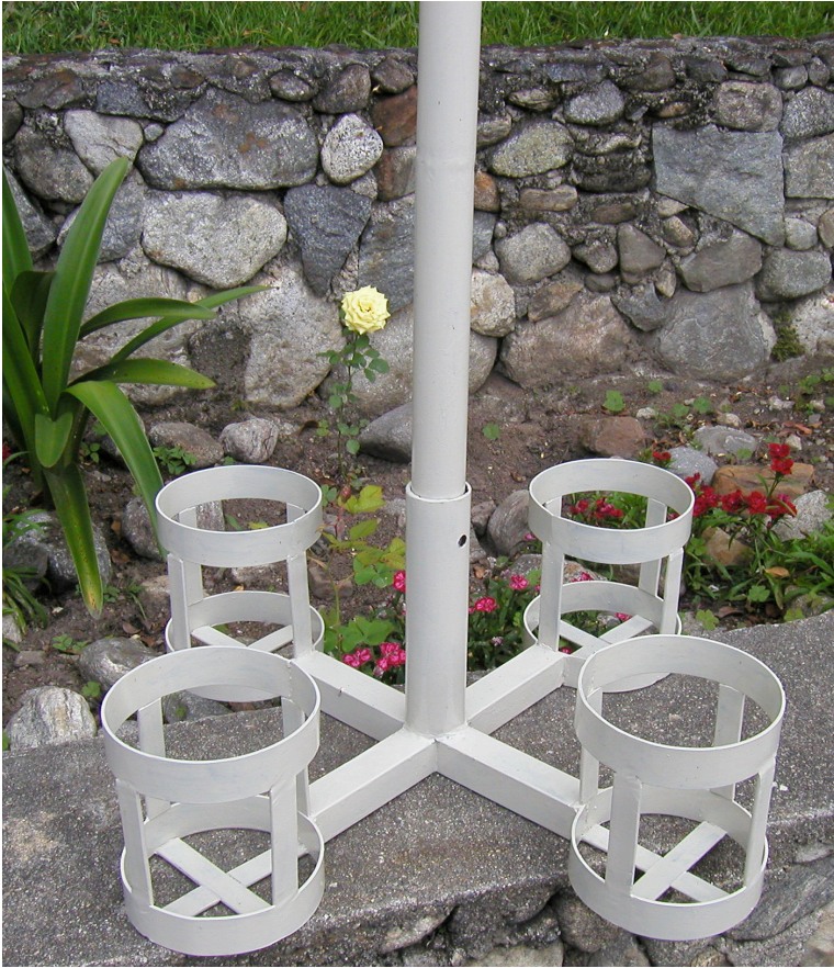
Figure 7.5: This metal base can be weighed down with sandbags, rocks, or water bottles to make a stable platform without penetrating a roof.
