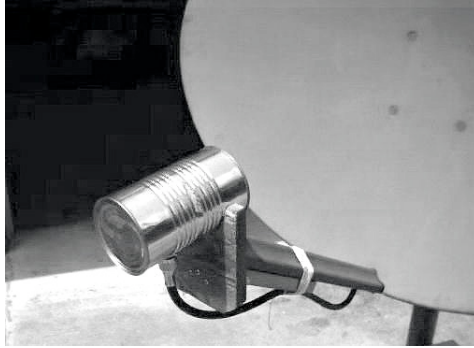
Figure 4.10: Feed horn made from a food can.
